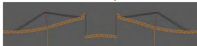
Figure 9: The lifting span operation results in a load balance that brings the bridge structure close to its final constructed profile.
