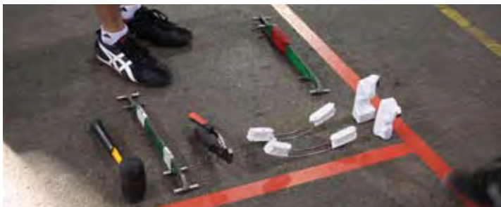
Above, below: The University of California at Davis design included several custom tools for holding members in place and making connections, shown below in the staging area and above in use during construction.
